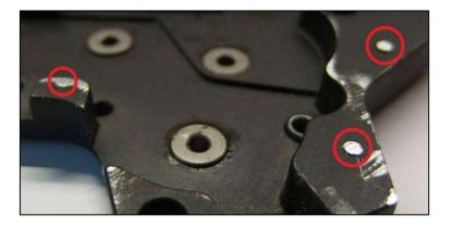
If your gearbox has high screw mounting, cut it off to flat surface.
