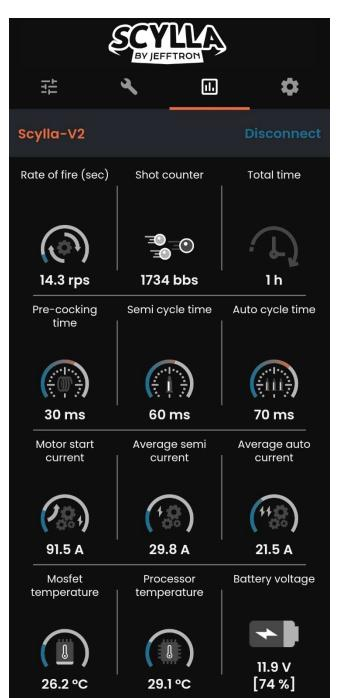
Motor start current: Peak current when the motor starts spinning.
