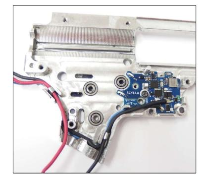
Wires to front: Red motor leads to the left hole and to the battery leads to front, it could be disconnected in the middle. Wires under the motor have to stick to the wall. You can use a hot glue to fix them to their position in the gearbox.
