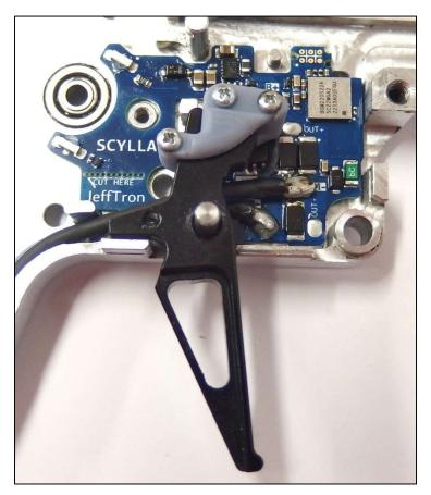
Check the sector gear height. Gear must not touch the optical sensor!
