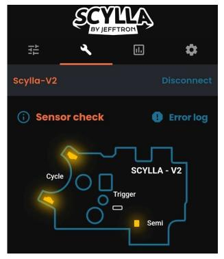
If any selector position ends in red, its value is too close to another one, so the position will not be set right.
