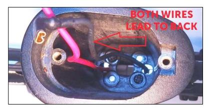
Connect the black wire first. Keep in mind the right motor polarity!
