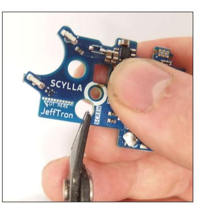
Put pliers near the drilled line and move the board up and down until it breaks of from the rest of the Scylla.
