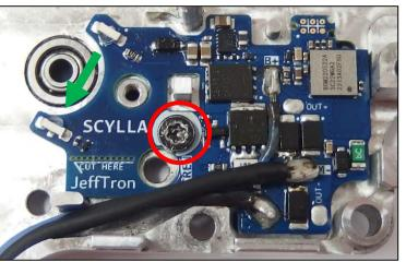
**too low**, move the sensor slightly **right** to be further from the sector gear or clean the sensor.
